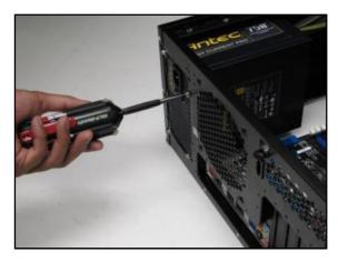
5. Re-attach the PSU support beam.
